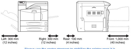
Always use the caster stoppers to stabilize the printer once it is in place to keep it from moving and/or falling over and causing injury.
